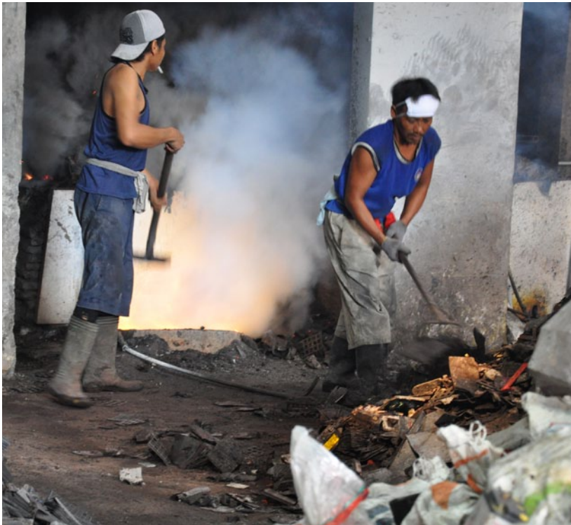
(Far left) A worker smelts or to extract lead in Bihar, India. Smelting involves the application of heat to mineral-rich rock or scrap metal to extract valuable metals. Health effects from exposure to lead via inhalation or ingestion include neurological damage, IQ decrement, anemia, muscle and joint pain, loss of memory, decreased concentration, nerve disorders, infertility, increased blood pressure and chronic headaches.
